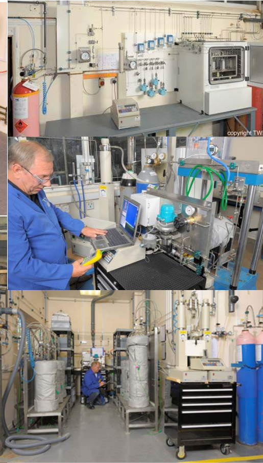
HPHT permeation, ageing and RGD testing of polymers
