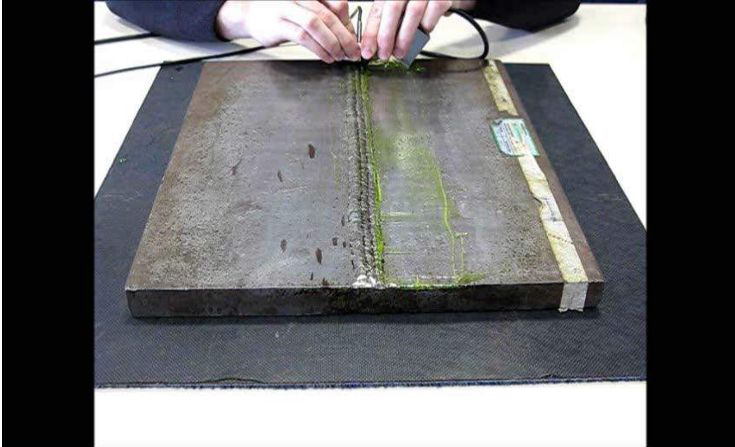
Double V-Butt weld 32 element probe + wedge
