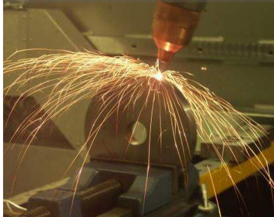
Nozzle powder delivery Laser Metal Deposition (LMD)
